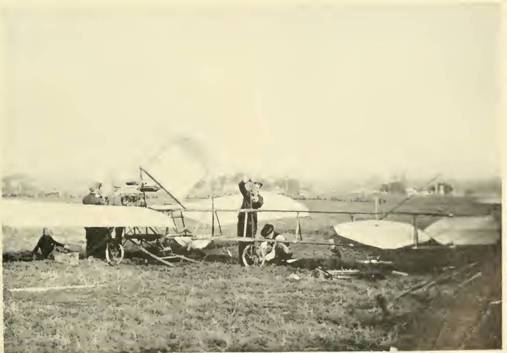
Klassen Monoplane (Lateral Balance By Hinged Fin)
