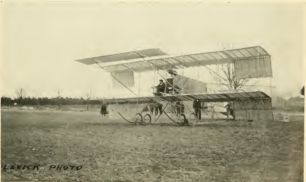
H. Farman Biplane—The Area of the Wing Tips has been Reduced Since the Above was Taken
