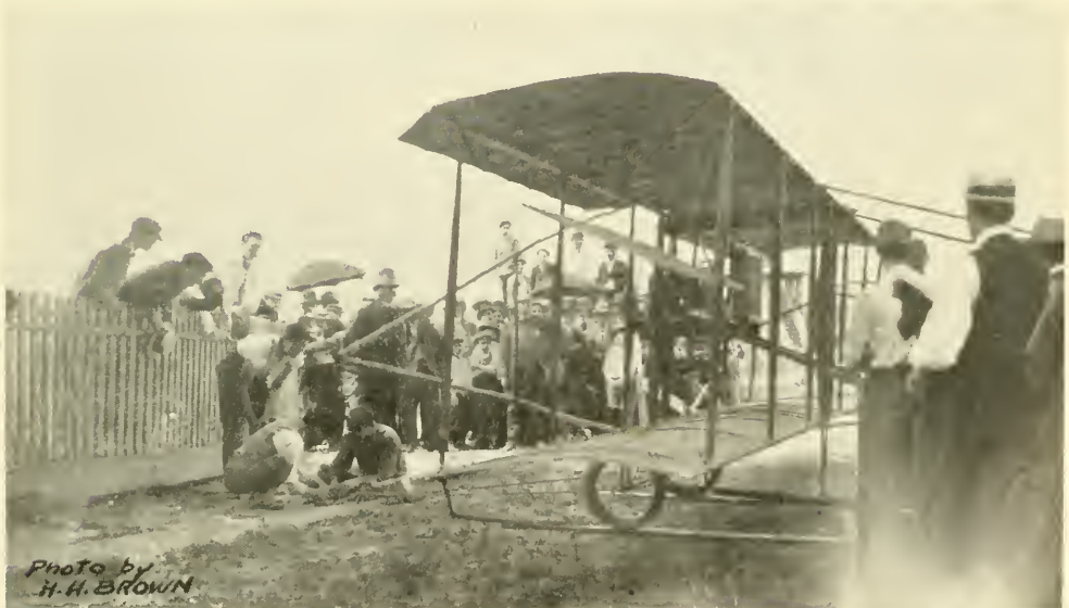
Testing Thrust on the Curtiss Machine — The Three to the Rear Are Noting the Pull On A Spring Balance
